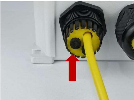
6. Fasten the clamping nut manually until it close the gap.
