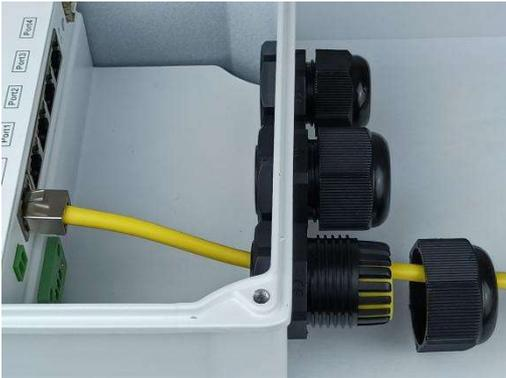
5. Repeat the step above to install the rest of the cable. Use rubber plug to block holes if you need some of them.
